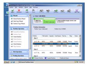
Step 2, Right-click the system partition and select "Resize", in the pop-up window, drag the right border rightwards to hold the Unallocated space.
